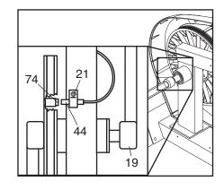
indicated M4 x 16mm Screw (21). Slide the Reed Switch slightly closer to or away from the Magnet. Then, retighten the Screw. Turn the Crank for a moment. Repeat until the console displays correct feedback. When the Reed Switch is correctly adjusted, reattach the left side shield and the left pedal.
